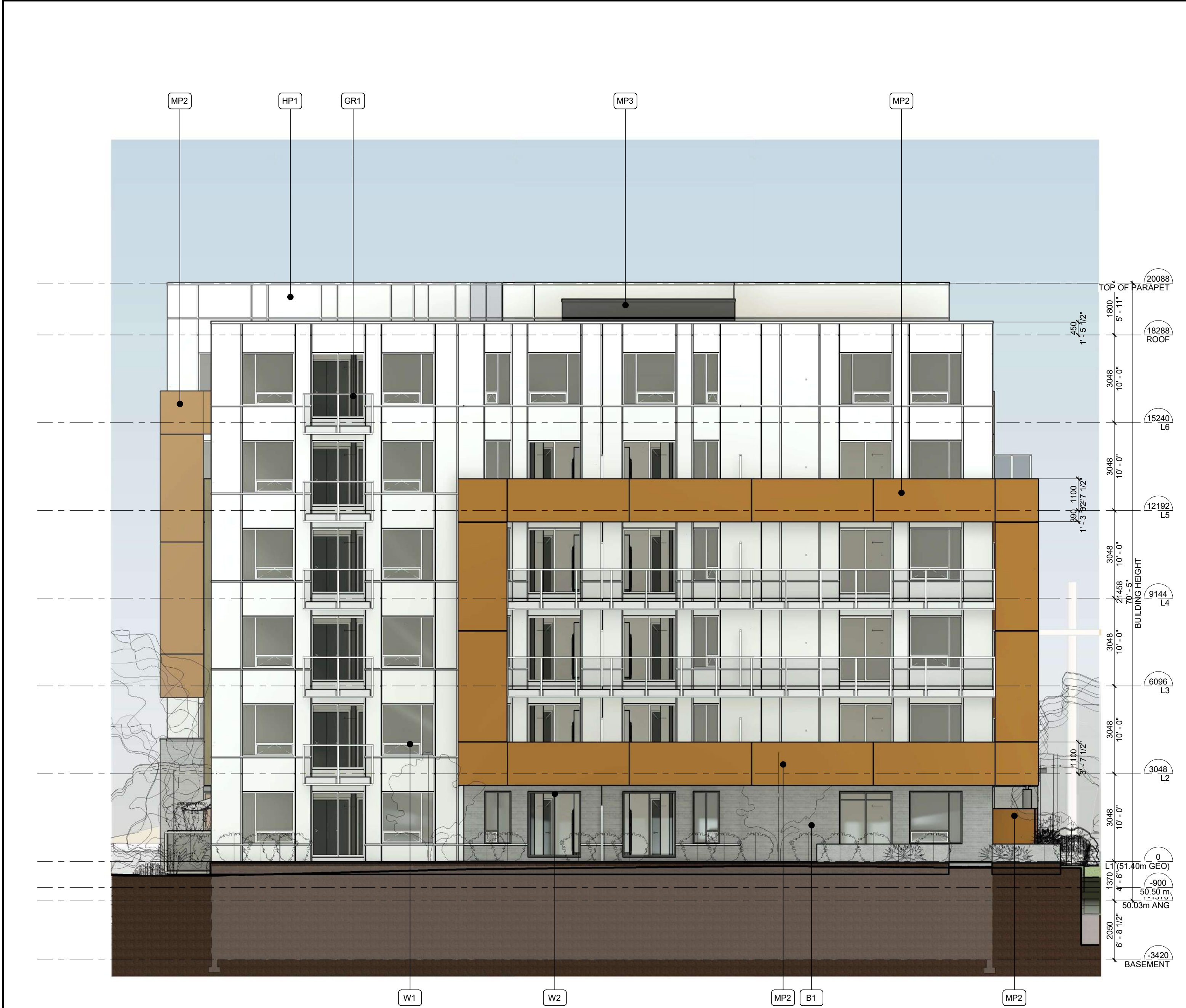
2 | EXTERIOR ELEVATION - NORTH 1 : 100 VISUAL SCALE 1:100 @ Arch D
