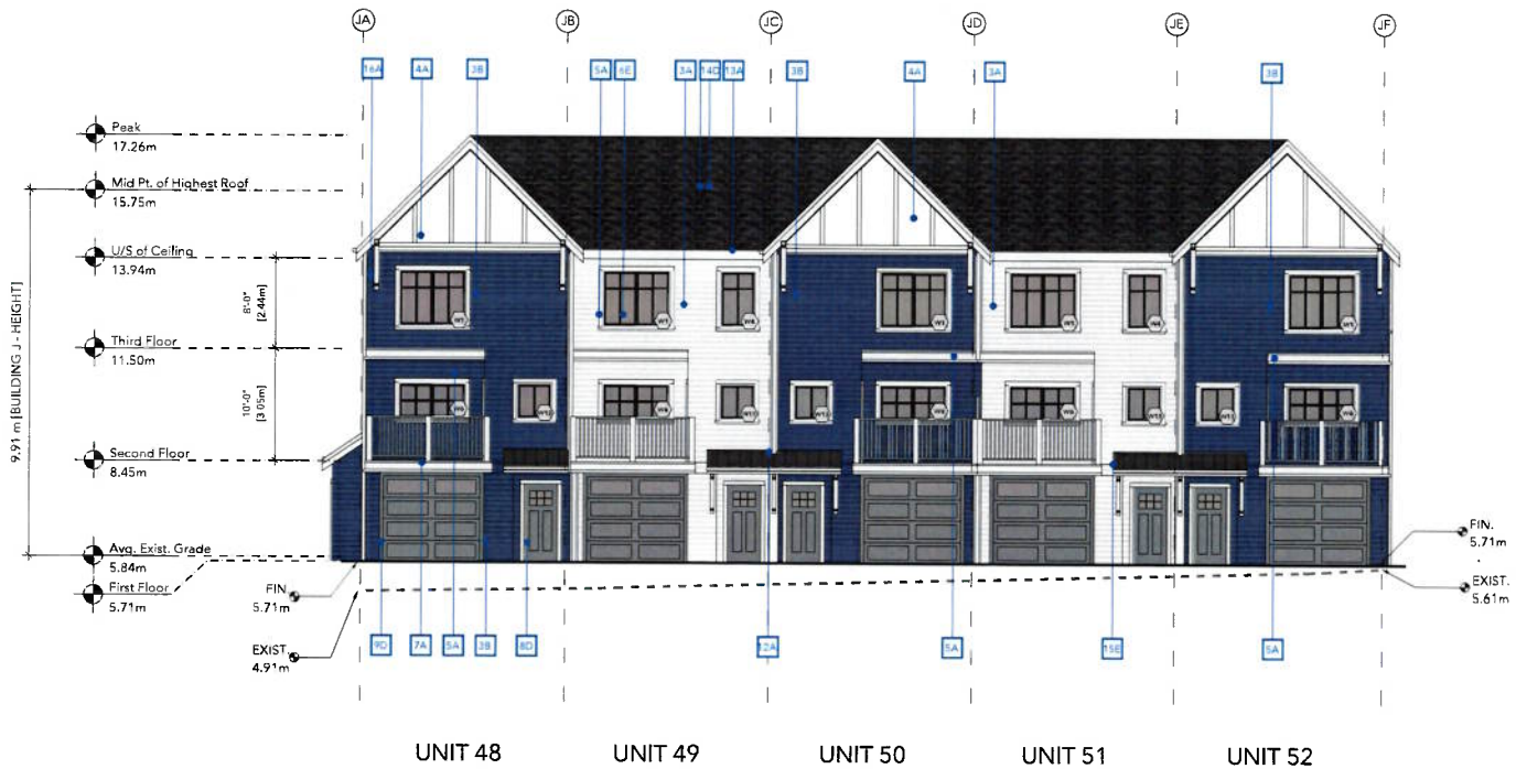
3 BUILDING J - SOUTH ELEVATION DP-28 SCALE: 1:100
