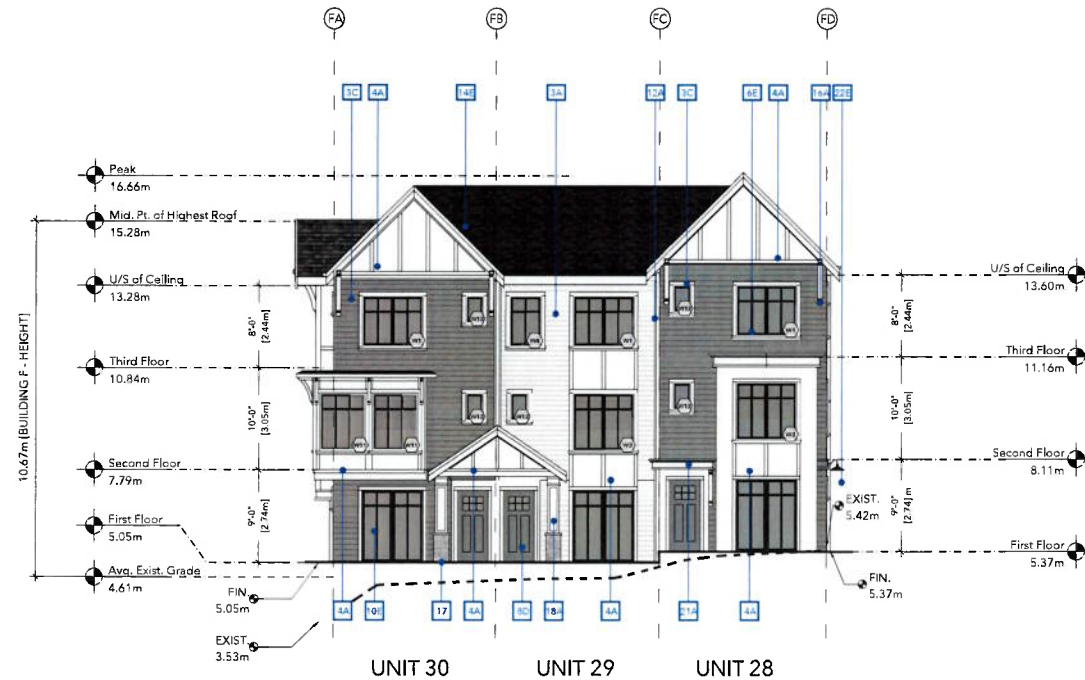
2 BUILDING F - EAST ELEVATION DP-24 SCALE: 1:100
