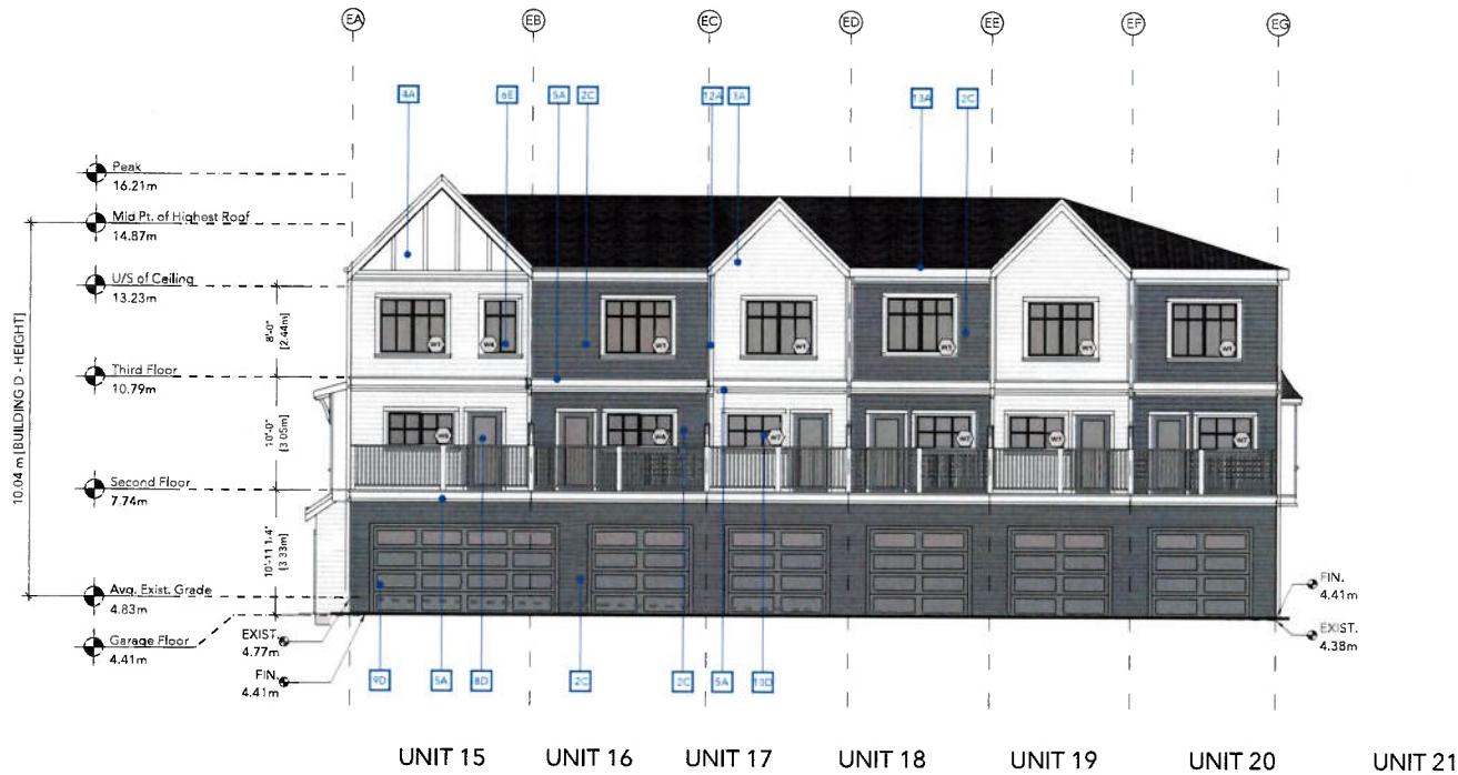
3 BUILDING E - SOUTH ELEVATION DP-23 SCALE: 1:100
