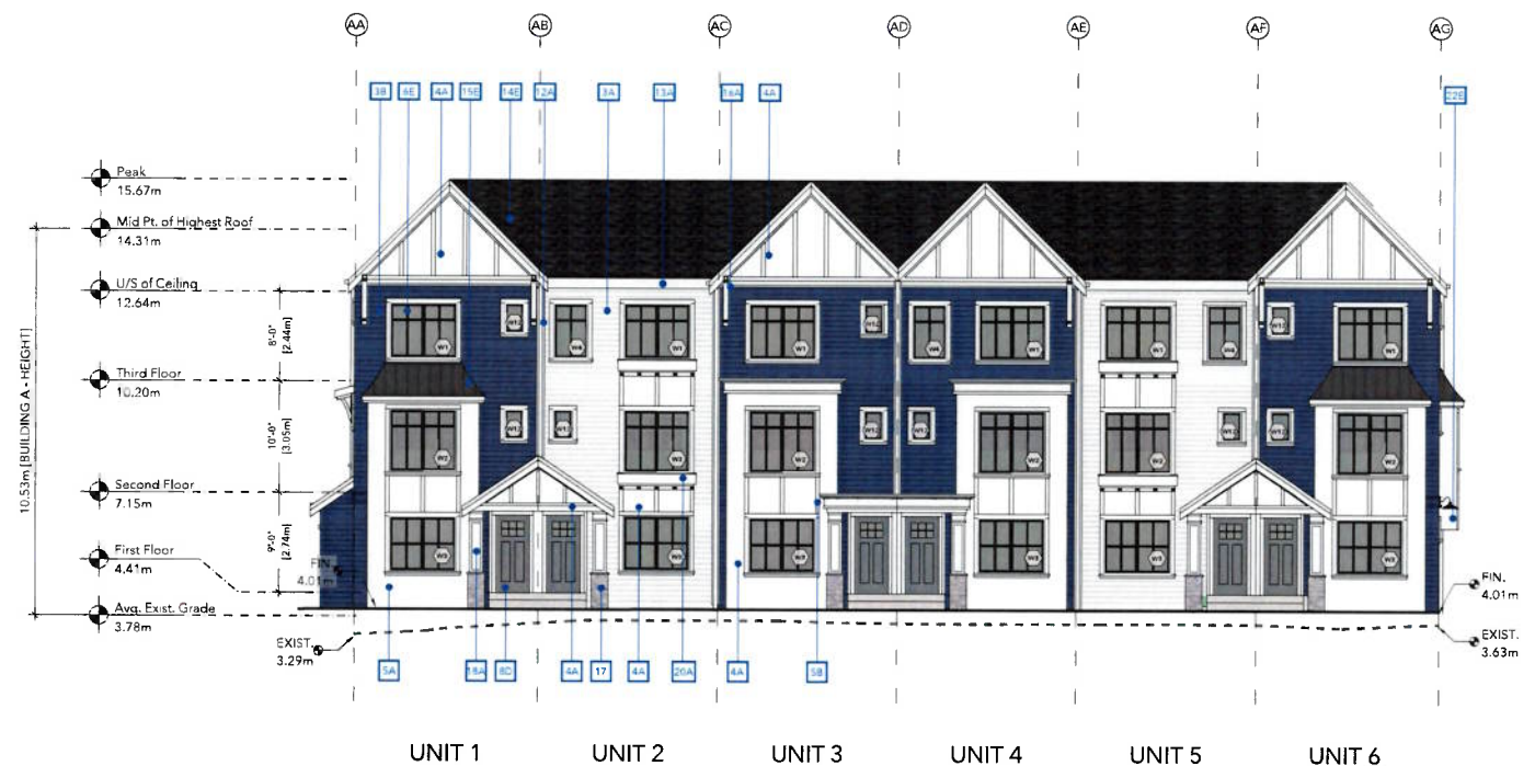
3 BUILDING A - SOUTH ELEVATION DP-19 SCALE: 1:100
