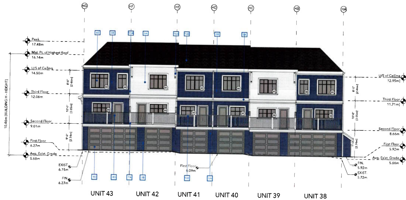
1 BUILDING H - NORTH ELEVATION DP-26 SCALE: 1:100
