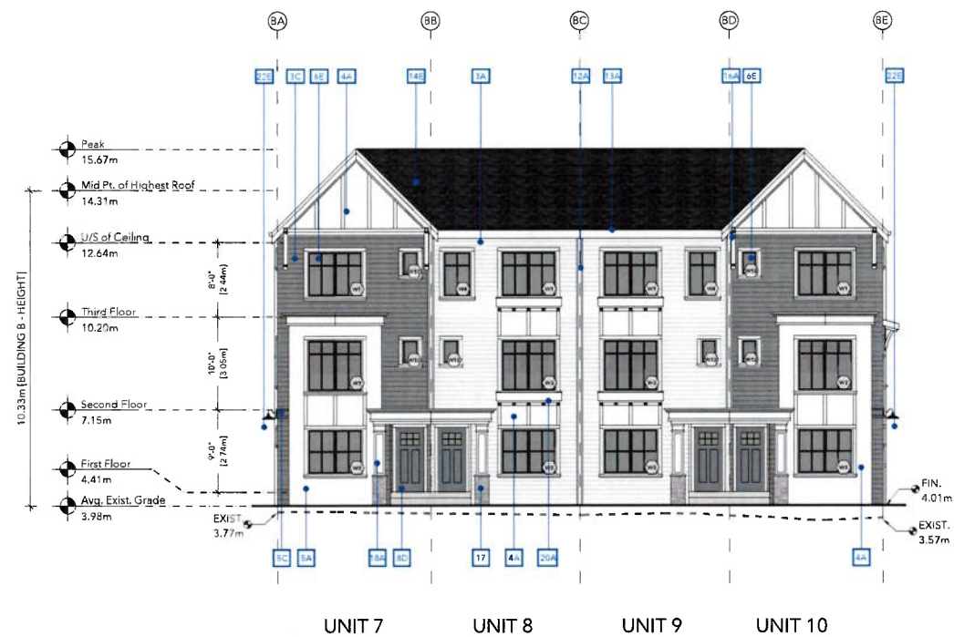
3 BUILDING B - SOUTH ELEVATION DP-20 SCALE: 1:100
