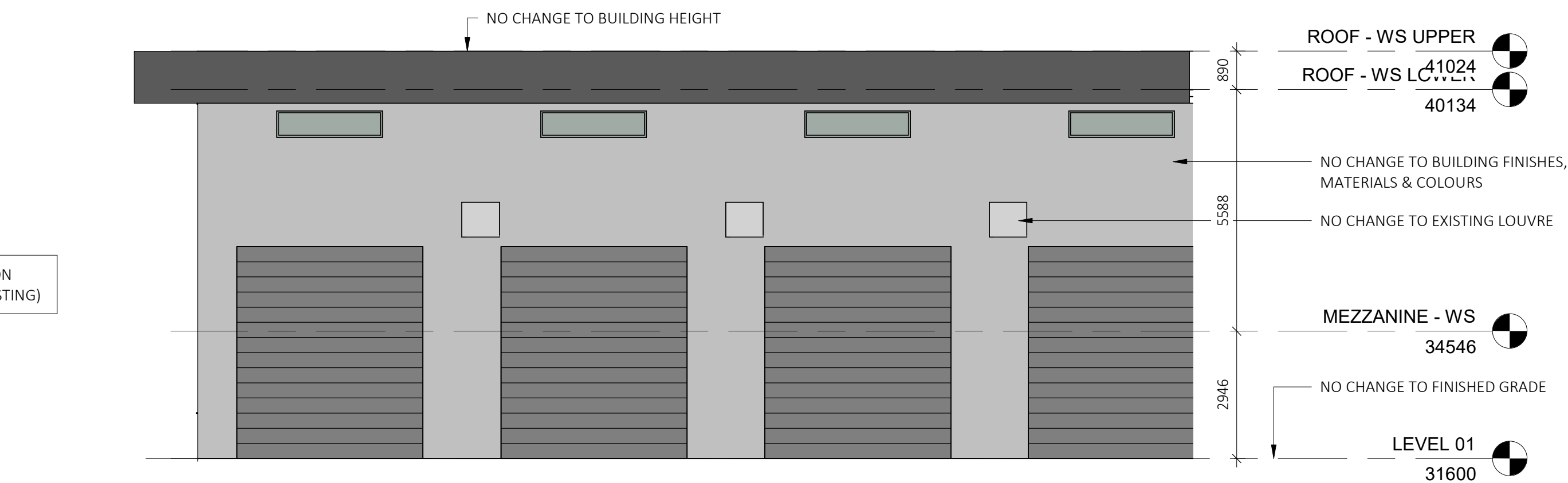
3 DP - WORKSHOP SOUTH ELEVATION 1 : 100
